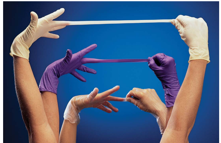
Three types of base glove materials (from top): natural rubber latex (NRL), acrylonitrile-butadiene (nitrile) and polyvinyl chloride (vinyl, PVC).
